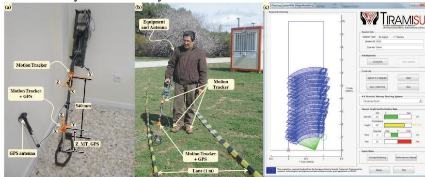
Fig. 1. (a) Compact metal detector with sensory system. (b) Apprentice with HHD training tool during an experimental test at CSIC premises. (c) GUI implemented in Matlab.
