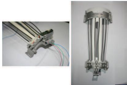
Figure 5 - ALAS actuating device
