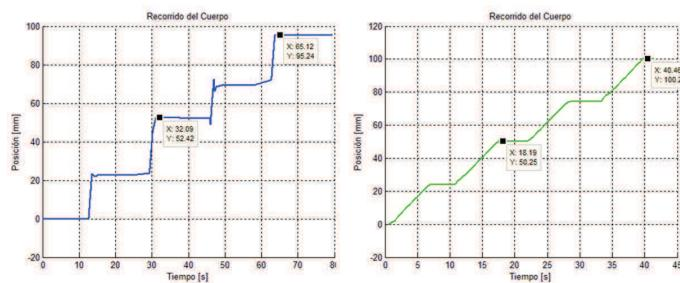
Fig. 6. Comparison between the motion of the robot during a discontinuous gait (to left) and continuous gait (to right).
