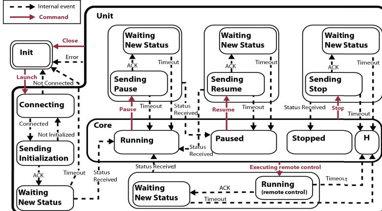
Figure 4. State diagram of the basic controller of a unit.
