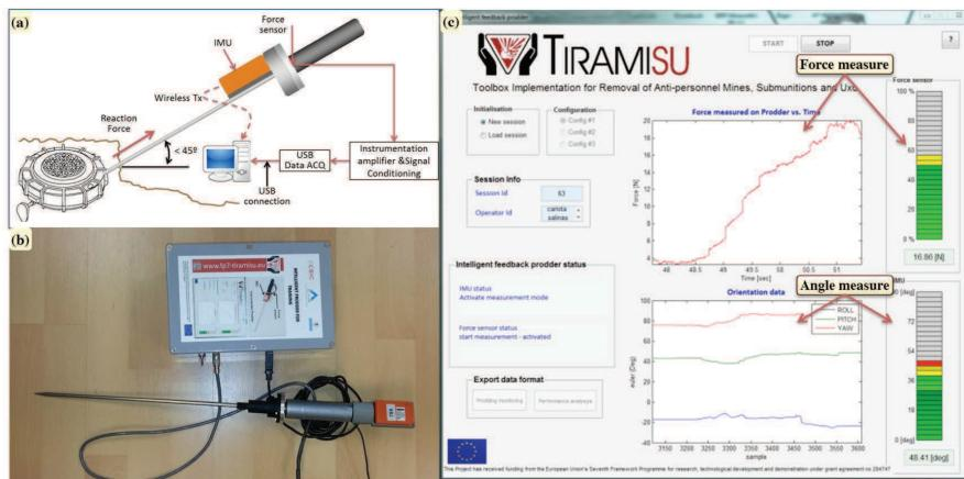
Fig. 2. (a) Block diagram of the intelligent prodder showing the different modules that compose it. (b) Intelligent feedback prodder (IFP). (c) GUI for the IFP.
