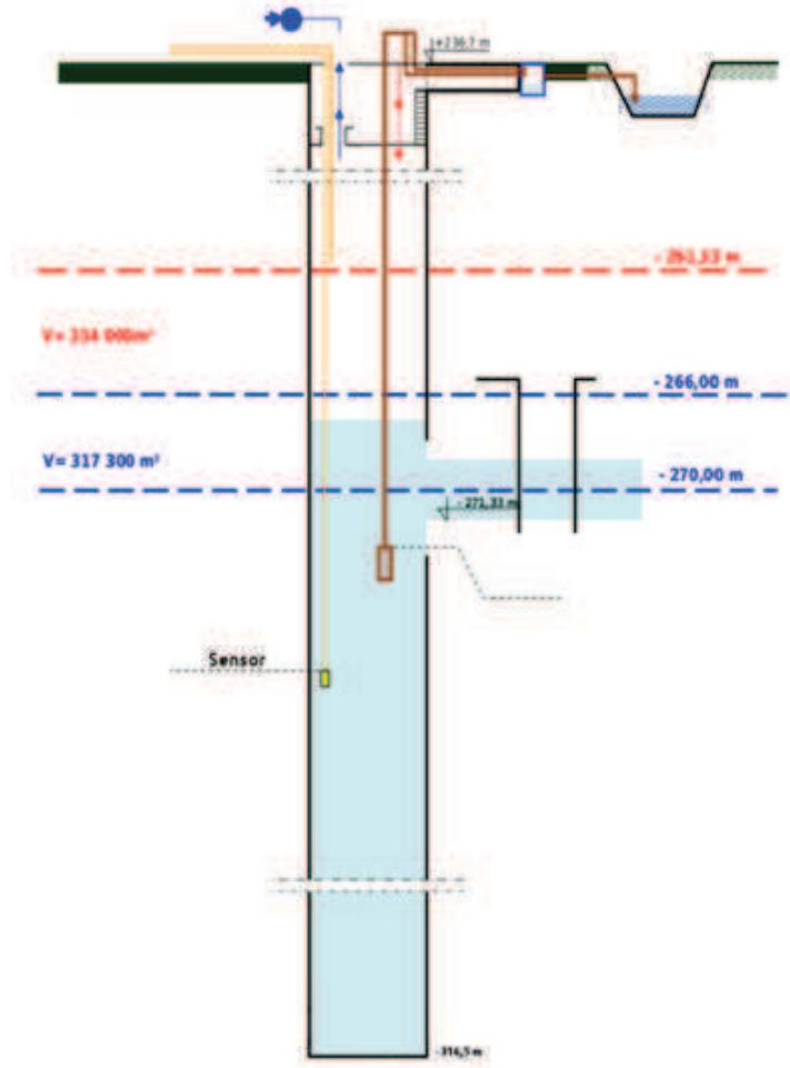
Figure 1. Typical flooded shaft with sensors
