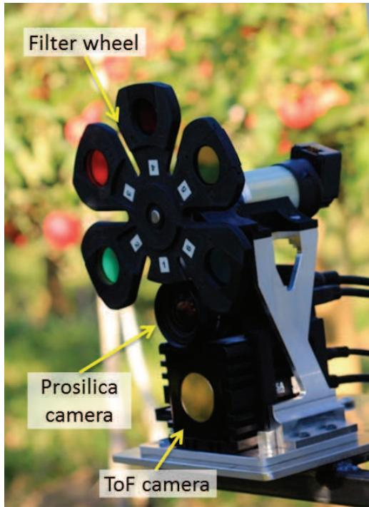
Fig. 1. Sensory system for detection and localization of fruits
