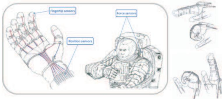
An important fact to be taken into account is that the demonstrator is intended to be integrated within an EVA glove. The device is light and low volume. The SMA wires are the basis of the actuating system, thanks to
