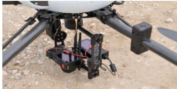
Fig. 2. Perception system on-board the drone
