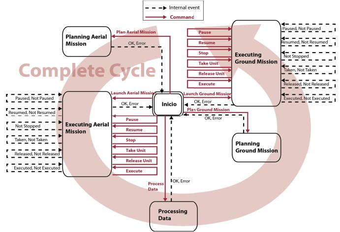
Figure 5. State diagram for the dispatcher.
