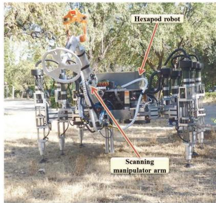
Fig. 5. Hexapod walking robot and scanning manipulator arm.
