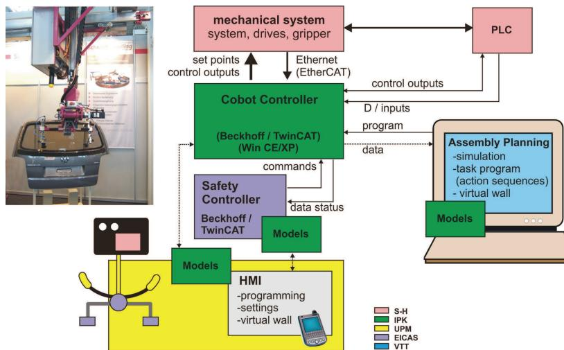
Fig. 4. Cobot control system architecture
