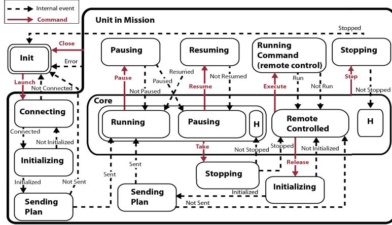
Figure 3. The state diagram of a unit controller for a mission
