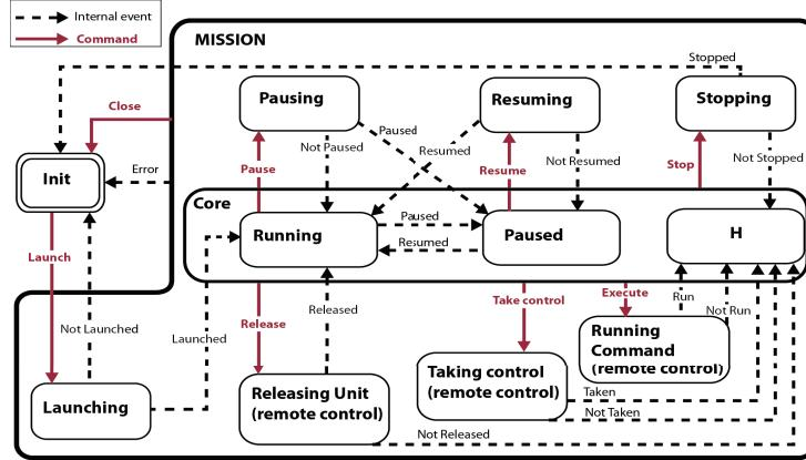
Figure 2. State diagram of a mission controller
