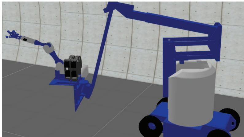
Fig. 3. Gazebo simulation of the ROBO-SPECT system
