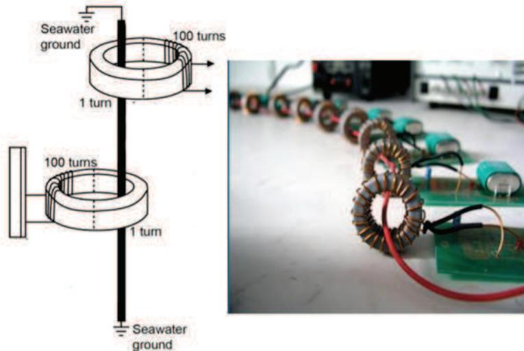
Fig. 4. Sensors with simultaneous power supply and communication
